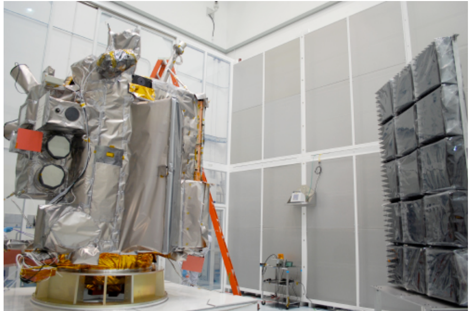
The RF absorber wall on the right is used during the Mini-RF testing.
