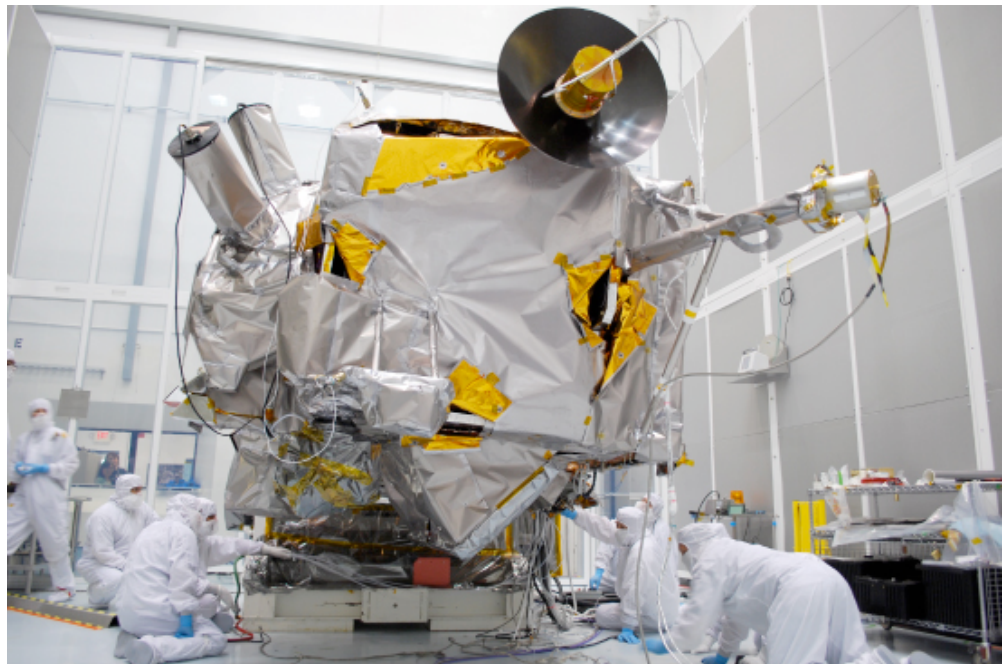
With the X-axis horizontal, we rotated to various positions for the blanket work. Here the team guides all of the cabling during a rotation.
