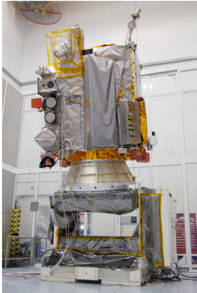
The Orbiter is on the turn-over fixture. We use this device to point the instruments toward the floor, so we can check the optical instruments.
