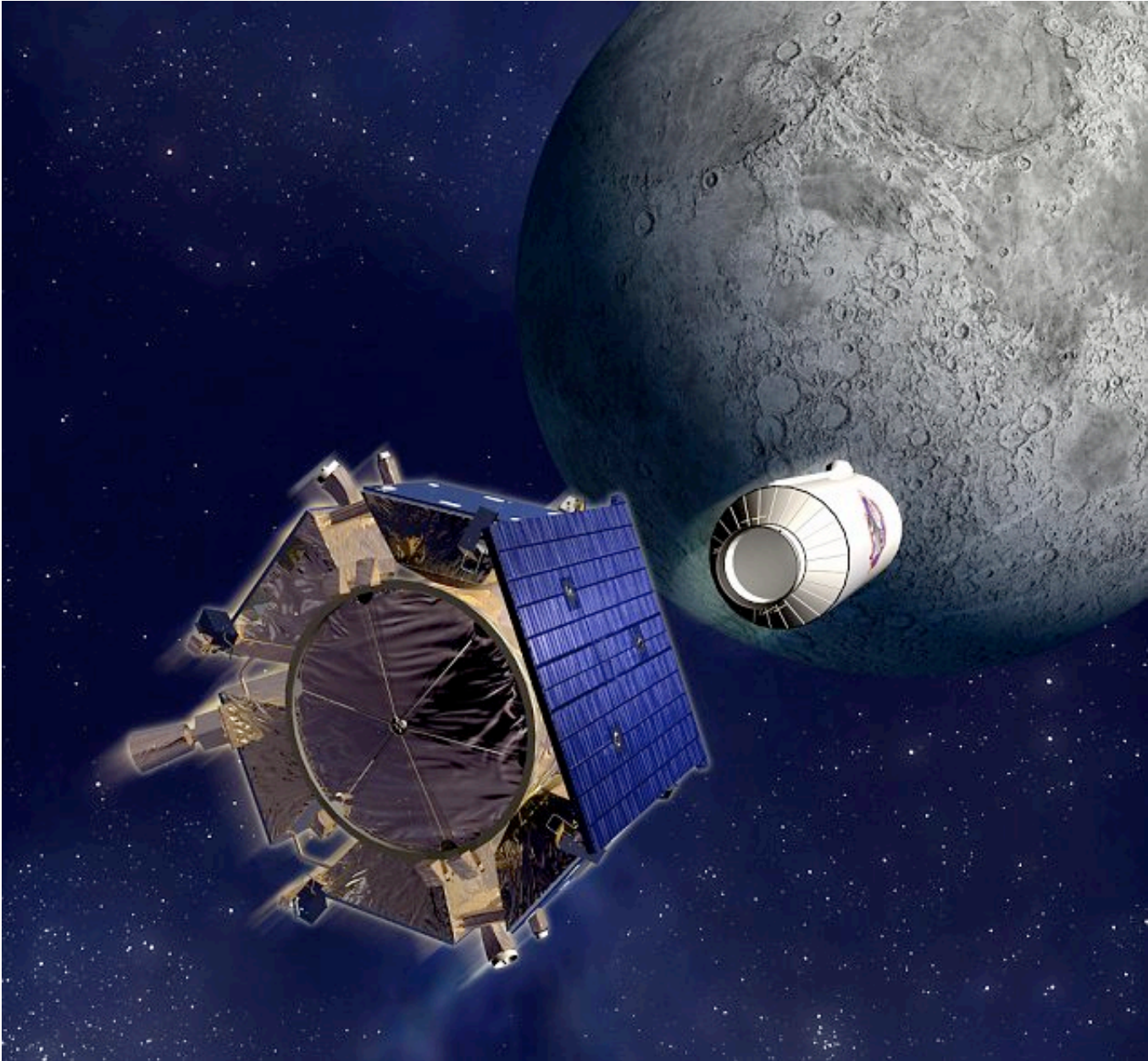
An artist's rendering of the LCROSS spacecraft and Centaur separation. The Centaur will make the first impact with the rest of the spacecraft passing through the debris plume four minutes later.
