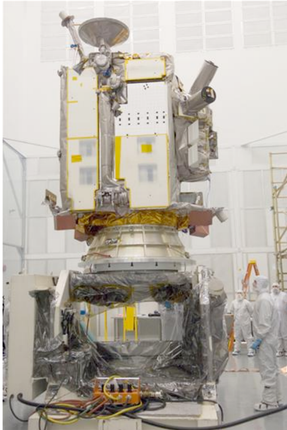
The Lunar Reconnaissance Orbiter sits on a testing platform in a clean room at NASA's Goddard Space Flight Center in Greenbelt, Md. This image gives an idea of the size of the spacecraft. Credit: NASA/Debbie McCallum
