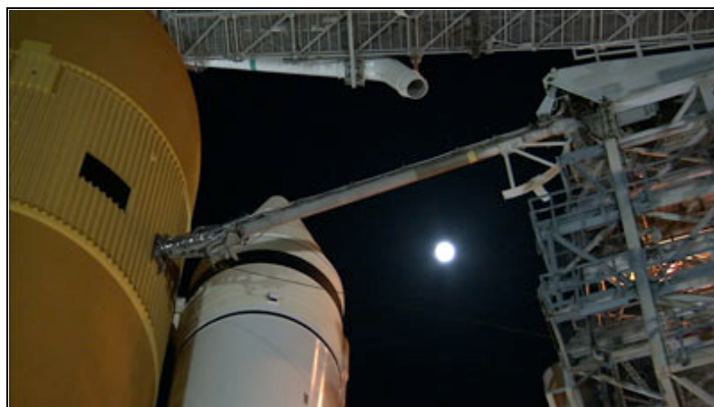
The file image shows the launch pad's gaseous hydrogen vent arm that connects the pad tower to the shuttle's tank. Credit: NASA TV
