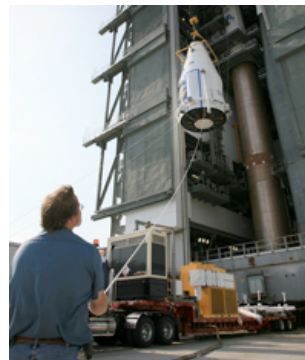
The Lunar Reconnaissance Orbiter, which contains a high-sensitivity camera, and the Lunar Crater Observation and Sensing Satellite are hoisted atop the Atlas V launch vehicle on June 17. Image: NASA
