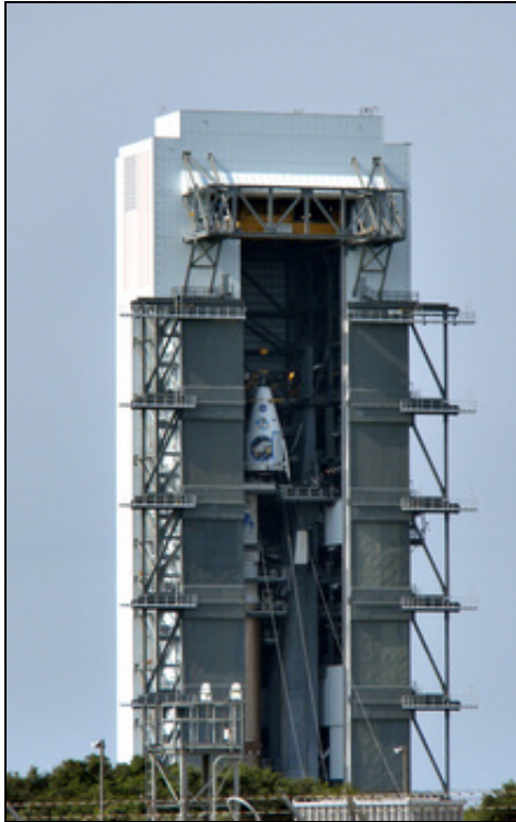
LRO being hoisted to the top of its Atlas V rocket.
