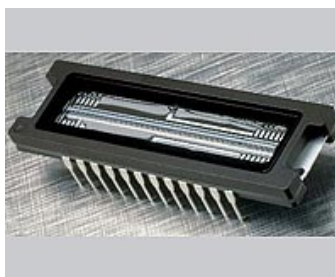
Two Narrow Angle Cameras on the orbiter will capture high-resolution images of the moon's surface at 0.5 meter-per-pixel using KODAK KLI-5001 Image Sensors (pictured), providing the same level of detail as the highest resolution satellite images of Earth commercially available today.
