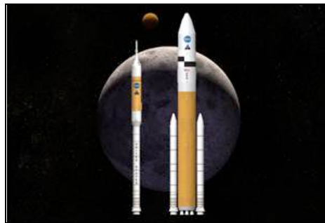
NASA An artist's conception shows the Ares I rocket at left and the Ares V rocket. The smaller rocket would be used for sending astronauts to orbit, and the larger one would carry cargo and
