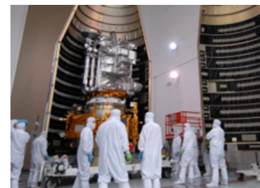
The LRO and LCROSS spacecrafts mated together and sitting outside of their rocket fairing. (Credit: Kennedy Space Center)
