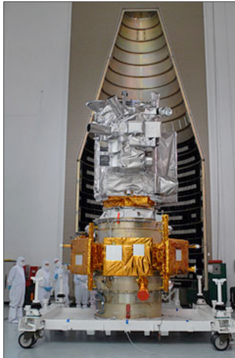
The LRO spacecraft sits atop LCROSS during final launch preparations. Credit: Ben Cooper/Spaceflight Now
