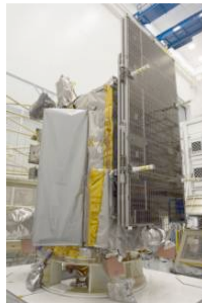
Here the Orbiter is on the Miller table undergoing mass properties measurements. We measure the mass, center of mass in two axes, and the moment of inertia in one axis. You can see the instrument module on the right. The radiator panel is the surface coated in mirrors. These Optical Surface Reflectors
