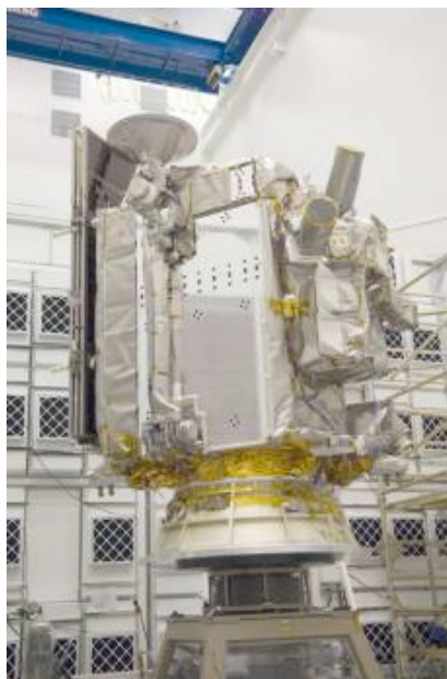
This view of the Orbiter shows the solar array on the right and the Mini-RF antenna on the left with the other instruments in the background. The bolt catchers sticking out from the array catch the hardware that keeps the array attached to the spacecraft during launch.
